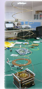
Antenna for ADS-B deployed
