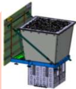
ECLAIRS , a 2D-coded mask imager
