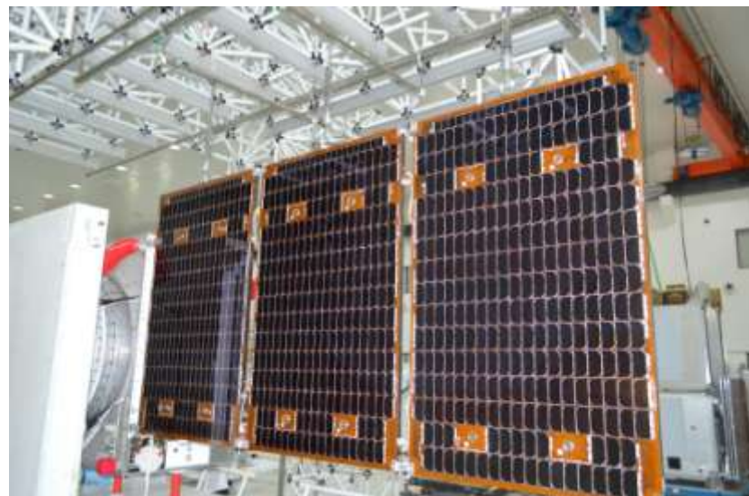
Solar panel deployment test
