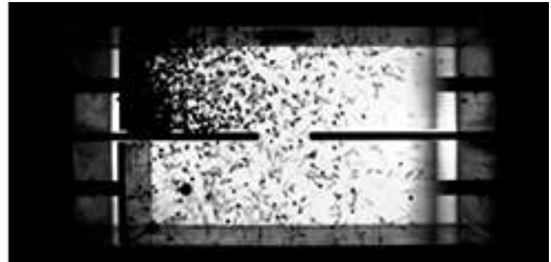
The obvious double bin separation imaged for the first time under microgravity conditions
